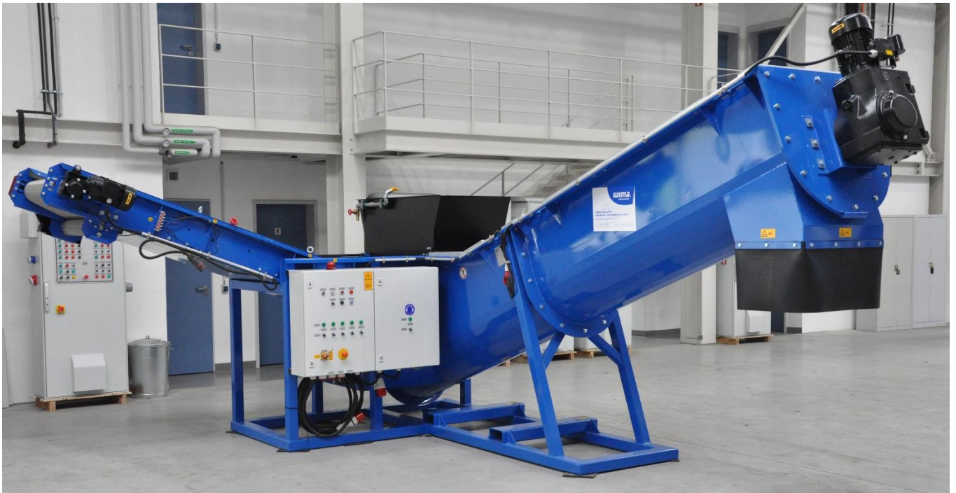
HDS-S view on auger, control cabinet and conveyor belt
